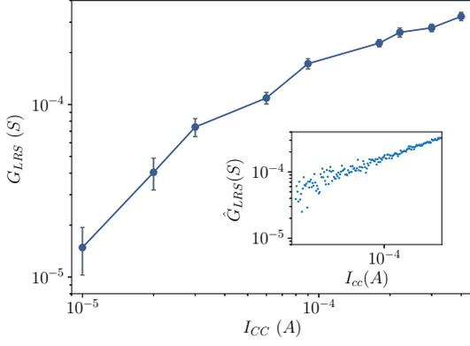
Fig. 1: Mean and STD of the device conductance as a function of the  $I_{CC}$ s. The inset shows the samples from the fitted mean and STD used for the simulations.
