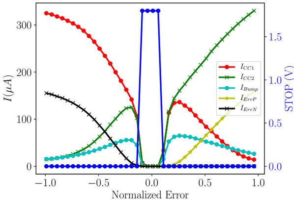
Fig. 4: Error current, STOP learning signal and  $I_{CC}$  as a function of the normalized error between the target and the neuron frequencies.
