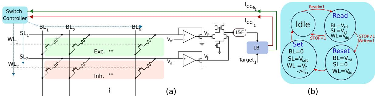
Fig. 2: Event-based neuromorphic architecture using on-line learning in a 1T1R array (a), and the asynchronous state machine used as the switch controller applying the appropriate voltages on the BL, SL and WL of the array for online learning.
