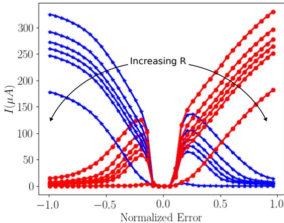
Fig. 5: Change of the  $I_{CC1}$  (red) and  $I_{CC2}$  (blue) as a function of the error and the resistance value of the devices.
