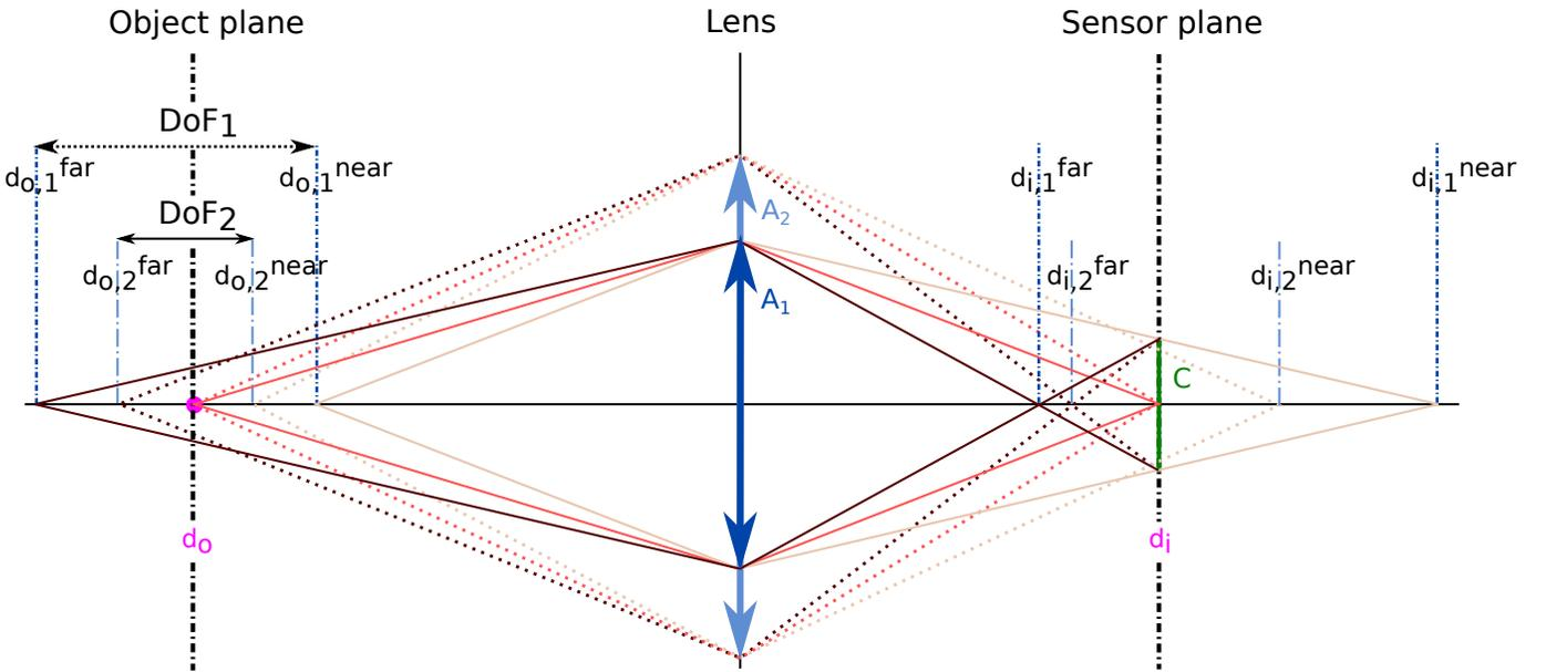
Fig. 2. An illustration of the depths of field  $DoF_{1/2}$  and the near/far limits of focus  $d_o^{near/far}$  for two apertures  $A_{1/2}$  using a convex-lens in front of a point. The size of a pixel on the image plane/sensor plane defines the circle of confusion  $C$  that sets the upper limit of resolution (Figure adapted from [6]).
