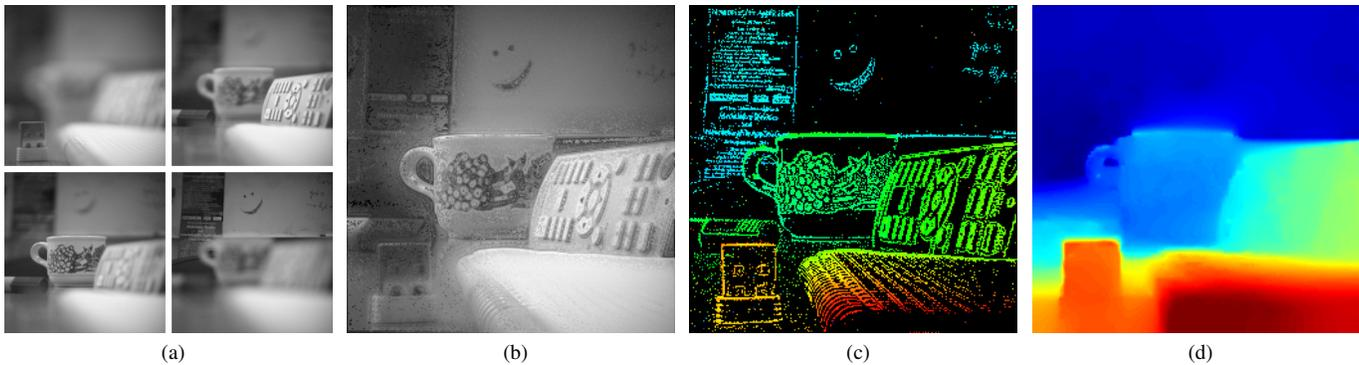
Fig. 7. An example scene imaged by our system: (a) shows four images extracted during a focal sweep illustrating the narrow  $DoF$  of our system; (b) shows an extended depth of field image (all points are in focus); (c) shows a depth map with 64 levels as captured by our system; (d) shows an inpainted, denoised and densified image as an example of post-processing that can be performed on images produced by our system.
