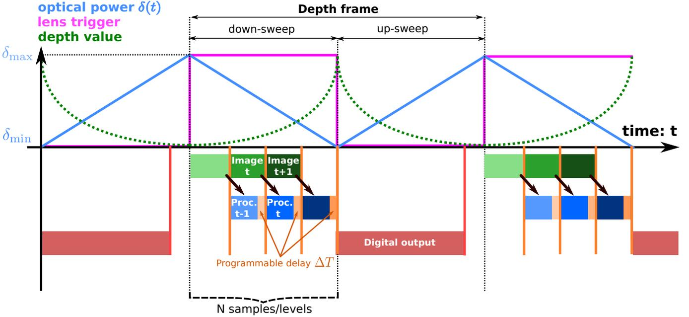
Fig. 5. A diagram illustrating timing in our depth from focus system and its pipelined imaging/processing operations.
