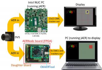
Fig. 1 Illustration of the two possible AER processing pathways of the demonstration: software-based (top) and FPGA-based (bottom).
