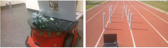
Fig. 1. The Dynamic Vision Sensor (DVS). Left) The DVS mounted on the Pioneer 2-DX robot Right) Experimental setup of 8 objects in open field covered with black/white checkerboard pattern.
