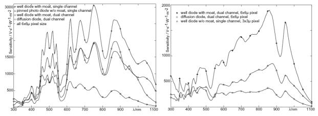
Figure 4: Spectral sensitivity of 90nm (left) and 65nm (right) photo diodes (30nm spectral gap width)
