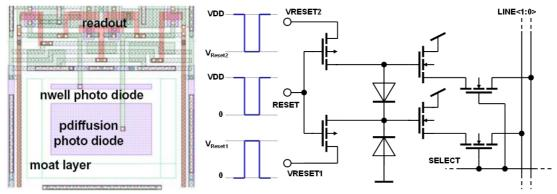
Figure 1: 6T dual channel pixel
