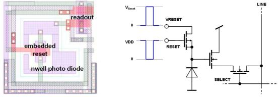
Figure 2: 3T pixel cell with embedded PMOS reset
