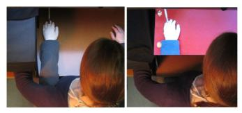
Figure 2. Rubber hand illusion test. (Left) Real rubber hand illusion, showing rubber arm being stroked with a paintbrush. (Right) Virtual rubber arm illusion, showing video of rubber arm being viewed in mirror.
