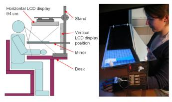
Figure 1: Mirrored arm display. (Left) Schematic of arrangement of mirror and monitor, showing the two possible positions of the monitor. (Right) Test subject wearing data gloves and viewing screen reflected in the mirror. The arms of the subject are lying on the table below the mirror. Due to the mirror reflection, the virtual arms appear to be level with the table.
