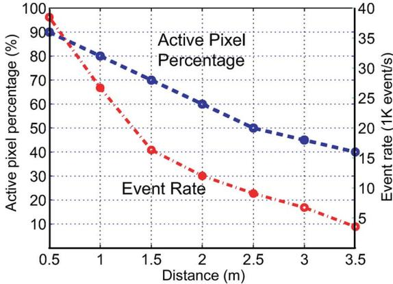
Fig. 10. Relation between (1) the event rate and the distance from the camera and (2) the percentage of active pixels and the distance. When the monitored person is 1 meter away from the detector, 80% of the active pixels in the sensor send events. In this situation, the detector cannot make accurate estimation of the motion centroid.
