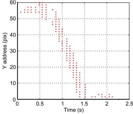
Fig. 5. Address-event responses from a frame-based temporal difference image emulator as it is tracking a free-falling object. The camera has a resolution of  $64 \times 64$  and runs at 30 frame/s. The imaged object is 3 m away and the camera is installed at 0.8 m. The uniform frame rate of the camera imposes a limit on the temporal difference sampling rate, which is 150 event/s on average.
