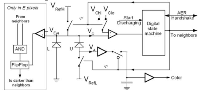
Fig. 3 Pixel architecture, including control state machine, sample and hold for the color value and the circuits for the computation of the eye feature (section C). The pixel consists of two photodiodes, two comparators, two source-followers, a capacitor and some digital control logic.
