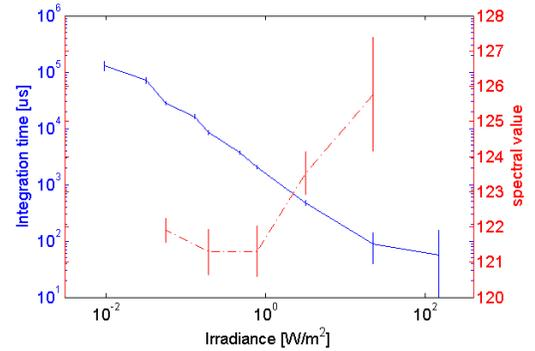
Fig. 5 Integration time (blue, solid) and 8 bit color value (dashed, red) vs. irradiance.
