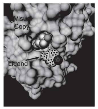
**Figure 8.** In the second experiment, when a ligand molecule (dotted atoms) passed through a configuration lower in energy than its current configuration during the exploration of the binding cavity, a visual copy of the ligand (shiny atoms) was displayed at that configuration to draw the attention of the subject.
