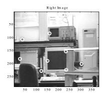
**Fig. 4.** Examples of matching target pairs denoted by white circles are shown. Here, the pan-tilt system was disabled and the algorithm searched for landmarks in static images.
