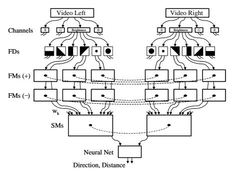
**Fig. 3.** From top to bottom: Each video image is split into four channels, each convolved with 6 FDs. The resulting 48 FMs on each side (only six shown here) serve as weighted stimulus for a SM that detects landmarks. The SMs provide input to a neural net estimating direction and distance to the landmark. Interactions between corresponding FMs belonging to the left and right stream and between the SMs are indicated by dotted lines.
