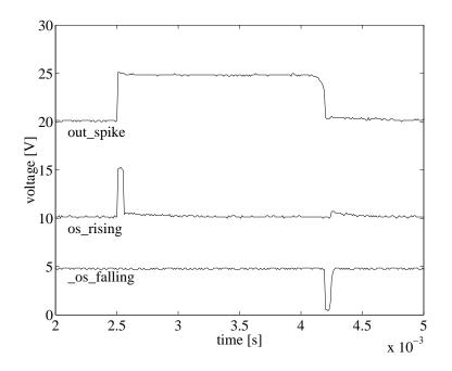
Figure 1.6 Scope traces of internal timing signals<sup>3</sup>, taken from a longer recording sequence. When  $os\_rising$  is high the weights get updated and then when  $\_os\_falling$  is low, soma and corr are reset. A presynaptic spike also produces a similar timing signal ( $ps\_rising$ , not shown here).  $ps\_rising$  allows synaptic current to flow to the soma and increments the correlation signal corr.
