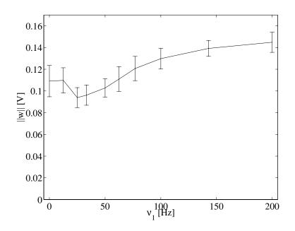
Figure 1.8 Again (see figure 1.7) the weight vector length for an experiment with two synapses stimulated with Poisson distributed spike signals is shown. This time the average frequency of synapse 2 is kept constant at 50 Hz. The x-axis shows the average frequency given to the other synapse ( $\nu_1$ ). The weights were taken as the mean of 200 oscilloscope traces of a duration of 200ms each. The bars show the standard deviation in these sets of 200 samples.
