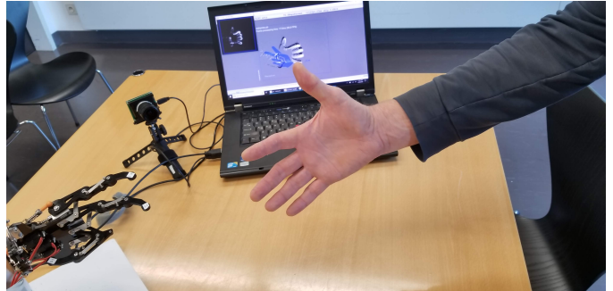
Fig. 1. “Dextra” robot hand driven by a convolutional network that can learn hand symbols on the fly.
