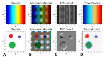
Fig. 2 Synthetic stimuli and responses. A: two synthetic stimuli: a rainbow varying sinusoidally in intensity in time and three moving color blobs. B: stimuli as seen by the silicon after color filtering. C: DVS histogram output (ON events are represented in white, OFF events in black and lack of events in grey), showing responses of the color DVS pixels. D: simple reconstruction [9].
