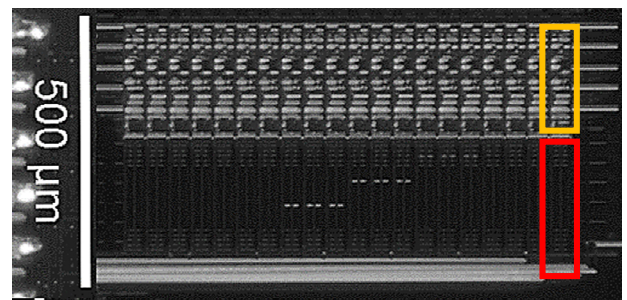
Fig. 3. Microphotograph of the array of AQC cochlear resonators (the rightmost filter's capacitors are highlighted in red and the circuit in yellow).
