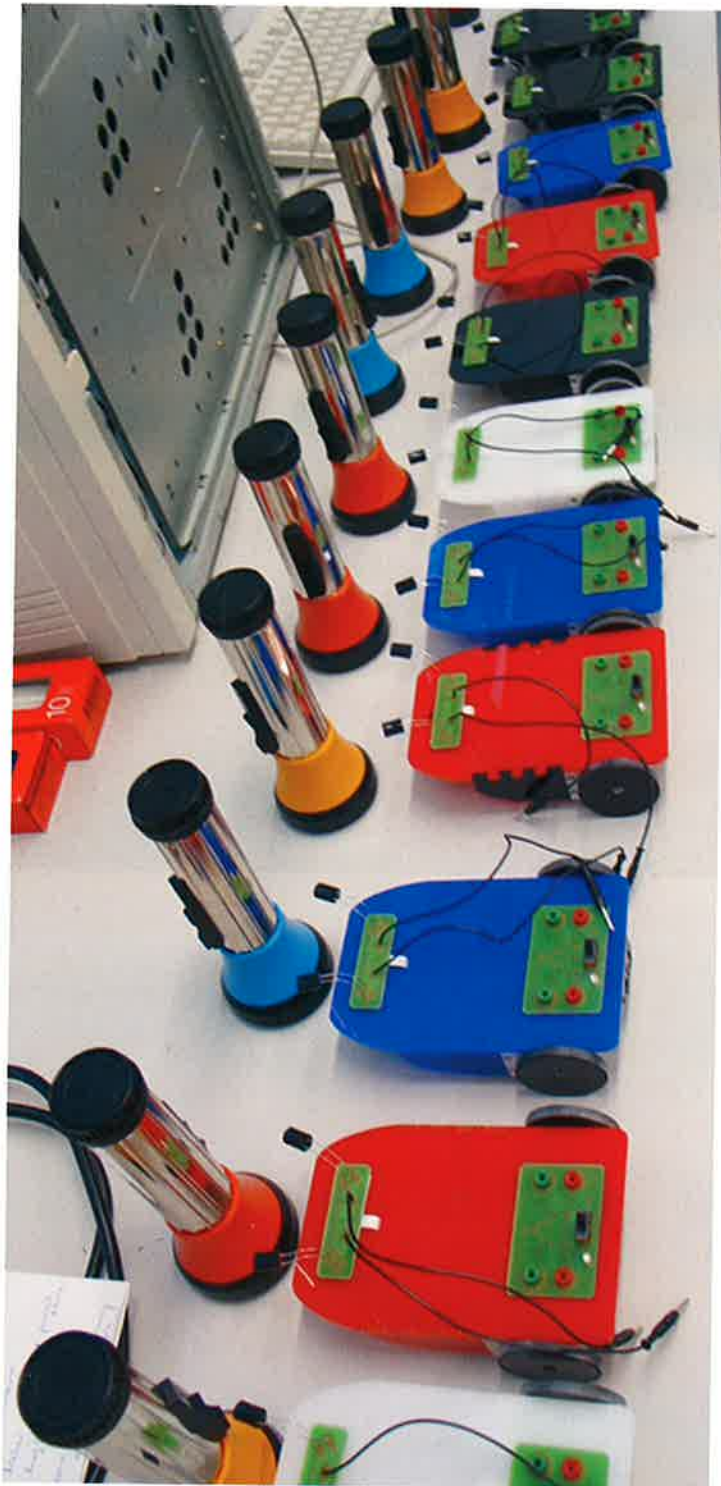
A platoon of Braitenberg Vehicles constructed by doctoral students at INI stand ready to teach school children the basics of neurorobotics.
