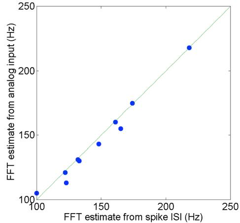
Figure 4. Data set of the 12 speakers (circles) showing that the fundamental frequency for a steady pitch computed from the FFT of the analog waveform vs the fundamental frequency computed from the ISI histogram.
