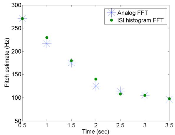
Figure 5. Data set of a speaker showing the correspondence for a time-varying pitch between the frequency computed from the FFT of the analog waveform and the frequency computed from the ISI histogram.
