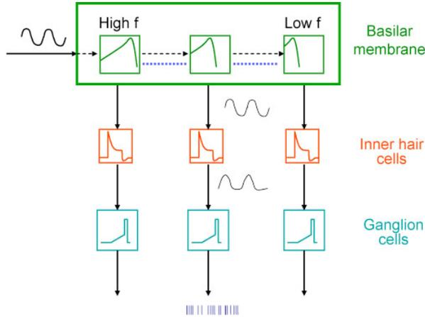
Figure 1. The block diagram of circuits of one of the 2 cochleas on the binaural AER EAR chip.
