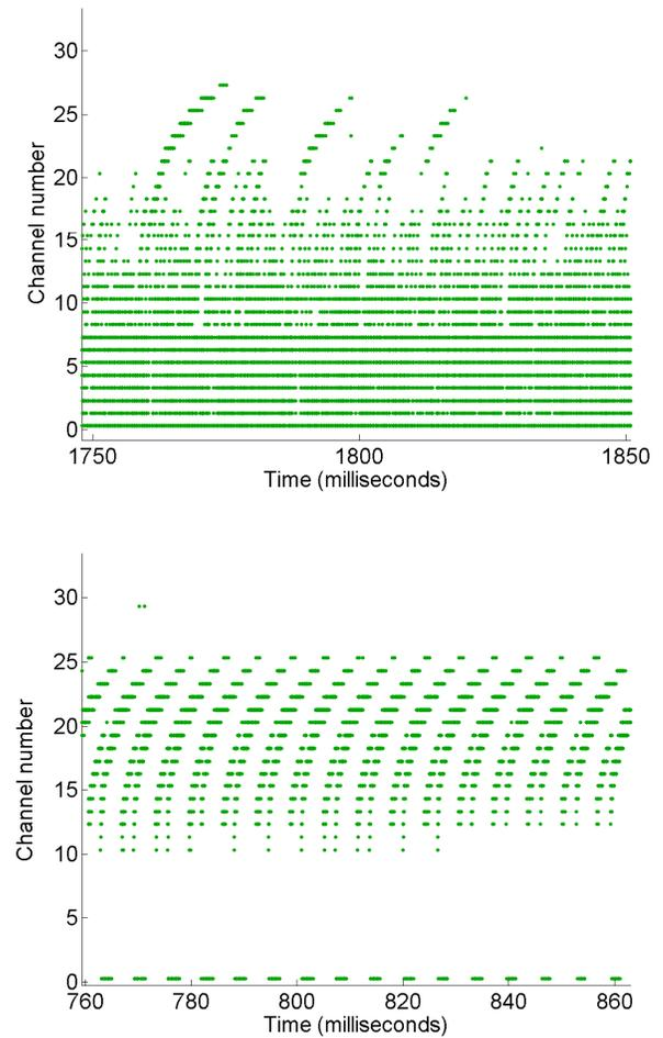
Figure 2. Spike responses from a single cochlea across 32 channels (y-axis) in response to (top) a “hiss” and (bottom) a “coo” from a speaker. Channel ‘0’ of this chip has a low threshold for spiking because of transistor mismatch.
