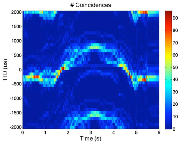
Figure 6. Localization data where a speaker voicing the “coo” sound moves continuously in time from the far end of one microphone to the other microphone and back again. The ITD is computed from the spike trains of the binaural cochlea.
