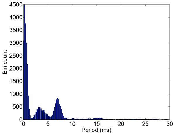
Figure 3. Histogram computed from 1<sup>st</sup> to 7<sup>th</sup> order ISIs of cochlear spikes from a single speaker voicing a “coo”. Peaks represent the harmonics in the speaker’s pitch except for the first peak which is due to the ISIs of spikes within a cycle.
