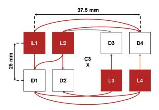
**Fig. 2.** Arrangement of light sources (L1, L2, L3, and L4) and detectors (D1, D2, D3, and D4) on the sensor. The centre of the sensor was positioned over C3. Ten channels were considered for analysis (red, one was measured twice (orange)), one was used to remove systemic physiological signals (grey).
