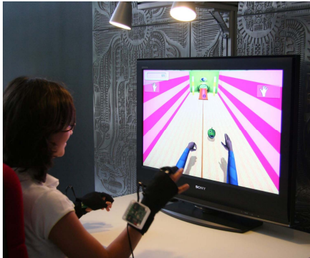
Fig. 2. The PITS system in use with a child. Shown are the monitor, table (100 x 60 cm) with adjustable lighting and wrap-around data gloves.
