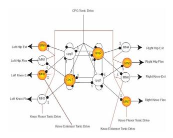
Figure 6. Typical CPG network for controlling Redbot [11]. The network is implemented with Integrated and Fire with Adaptation neurons (IFA). The neurons are connected to realize half-center oscillators for hip control. Knee muscles are 90 degrees out of phase with the hips, which is realized also using mutual inhibition.
