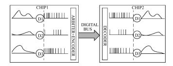
Figure 1. Rate-Coded AER inter-chip communication scheme.
