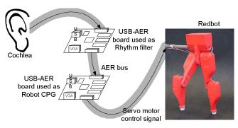
Figure 2. Block diagram of the experiment. A silicon cochlea is connected, via an AER bus, to a USB-AER board implementing a rhythm filter, which in turn is connected to another USB-AER implementing the redbot CPG that generates the servo motor control signal for the Redbot.
