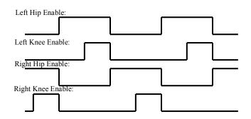
Figure 7. Servo enables for Redbot walk CPG.
