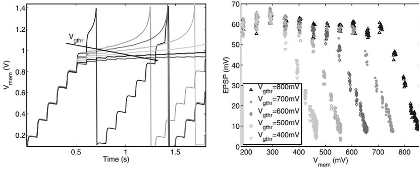
Figure 9: Conductance-based synapse. (Left) Membrane potential of the I&F neuron stimulated by the synapse for different values of the synaptic reversal potential  $V_{gthr}$ . (Right) EPSP amplitude as a function of  $V_{mem}$  for different values of  $V_{gthr}$ .
