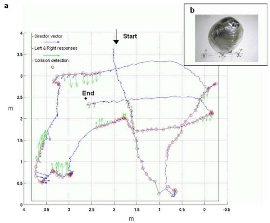
**Fig. 6** (a) Trace describing one minute of free flight of the UAV with both stabilization and collision avoidance systems enabled. Blue trace: the position of the UAV every 200 ms. Green arrows: the direction of the compensation responses to detected drift. Red dots: collision detection. (Adapted from Bermúdez i Badia et al., 2005) (b) Indoor UAV blimp platform. A mylar blimp filled with helium is propelled by 4 geared DC motors (motor: 08GS61-107.7 with gearbox 4:1 R10.0.4 both from
