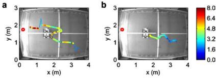
Fig. 14 Chemical search behavior of the robot in an environment containing obstacles using the LGMD-based optomotor collision avoidance system. (a) Trace of the robot with the obstacle avoidance module switched on. The robot is able find the odor source. (b) Control trace with the obstacle avoidance module switched off. An obstacle was placed in the wind tunnel (box at position  $\sim$  (1.5 m, 1.5 m)). The ethanol source is denoted with a red circle. The detection of imminent
