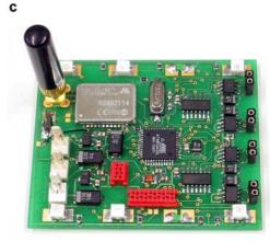
**Fig. 3** Experimental setup. (a) The robot setup and its communication with a ground station. See text for further explanation. (b) Diagram of mobile robot control and sensor integration modules. See text for further explanation. (c) Mobile robot control board using a Bluetooth Class I communication module (range up to 100 m). Weight: 23.5 g, dimensions:  $56 \times 67 \text{ mm}$
