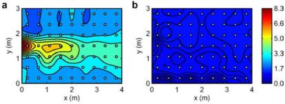
**Fig. 9** Wind tunnel calibration using static measurements of ethanol. (a) Response to a 9.4% solution of ethanol in distilled water. (b) Response to distilled water only (control). The response was sequentially measured using a single sensor placed for 2 min at 9 times 7 equally spaced locations (white dots). The obtained map of time-averaged sensor responses (window size 2 min) was smoothened (bi-cubic filter) and
