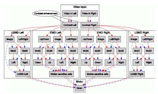
**Fig. 8** Block diagram of the collision avoidance and course stabilization model used for controlling the UAV. Each block indicates one population of simulated neurons. Red arrows represent excitatory con-
