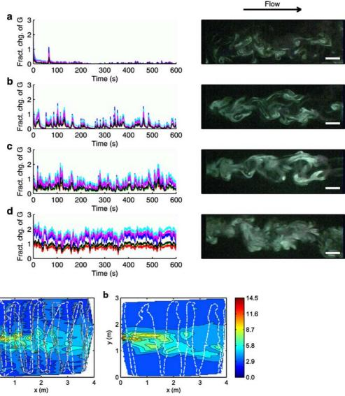
**Fig. 11** Dynamic response map. Spatial distribution of the responses of the chemosensor while moving through the wind tunnel (a) averaged over three runs and (b) computed from a single run. The dashed lines indicate the track of the robot. The odor source was located at (x, y) = (0 m, 1.5 m). For illustration purposes, the chemosensor response between
