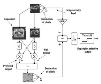
Fig. 5 Implementation of the LGMD model, making use of the Reichardt correlator (Reichardt, 1961), where  $\delta$  represents a delay, "×" the multiplication and "-" the subtraction operation. This model responds to looming stimuli in the visual field normalizing the strength of the response with the global activity level of the image using feed forward inhibition. The specific and non-specific inputs are integrated over time and thresholded (adapted from Bermúdez i Badia and Verschure, 2004)
