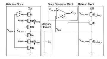
Fig. 4. Schematic diagram of the plastic synapse. The internal state of the synapse is determined by the voltage across capacitor  $C_s$ . The state generator block and the refresh block ensure the preservation of memory on long time scales. The Hebbian block contains all the information about the learning prescription. See the text for more details.
