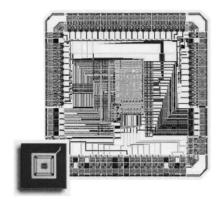
Fig. 1. Layout of the chip. It is a  $3.16\times3.16~\text{mm}^2$  chip implemented using standard  $0.6~\mu\text{m}$  three-metal CMOS technology.
