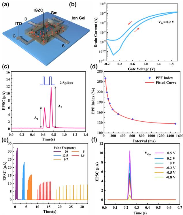
Fig. 3. (a) Schematic diagram of the synaptic transistor. (b) Transfer characteristic. (c) Typical PPF phenomenon. (d) PPF index as a function of spike time interval. EPSCs under spikes with various frequency (e) and  $V_{Gm}$  (f).
