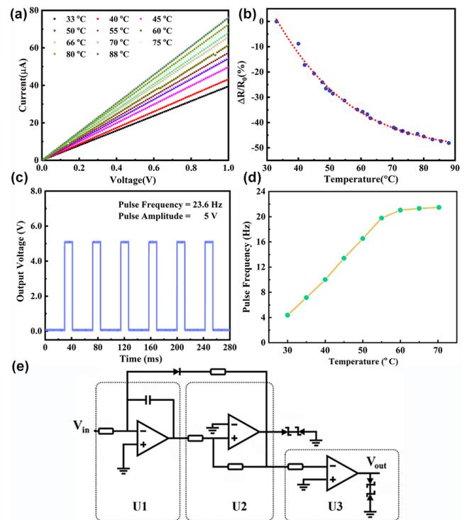
Fig. 2. (a) I-V characteristics of the temperature sensor. (b) Normalized resistance changes as a function of temperature. (c) A typical encoded spiking sequence. (d) The frequency of encoded spikes as a function of temperature. (e) The circuit diagram of the spiking encoder module.
