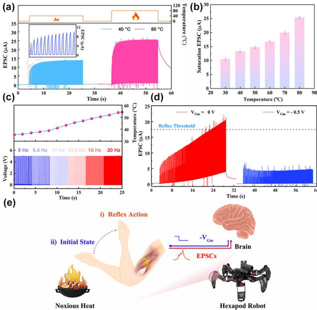
Fig. 4. (a) EPSCs generated at 40 and 80 °C. (b) The saturation EPSC under various temperatures. (c) Spikes generated from the encoder from 35 to 55 °C. (d) EPSCs under dynamic thermal stimuli by applying various  $V_{Gm}$ . (e) Working mechanism of an implanted artificial nerve.
