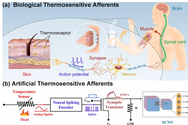
Fig. 1. (a) Schematic of the biological thermosensitive afferents. (b) Schematic diagram of the artificial thermosensitive afferents.
